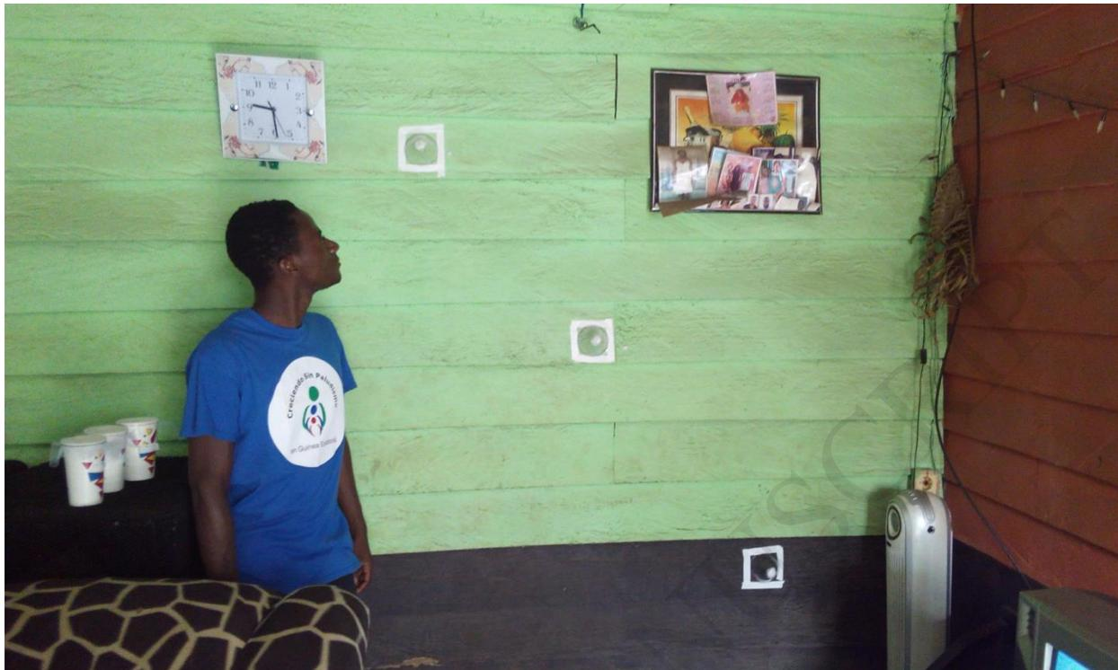
Fig.1. Standard WHO cone bioassay with Fludora™ fusion insecticide on wooden surface on Bioko Island (Colour print is needed for this figure).
